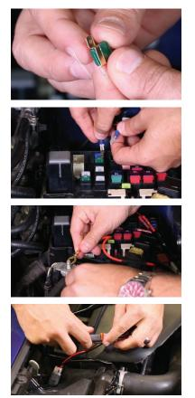
5. Install the included spade connectors onto both fuses. To do so, line up the slot with one of the spades on the fuse and slide the spade connector over to lock it into place. Repeat the process for the other fuse.
